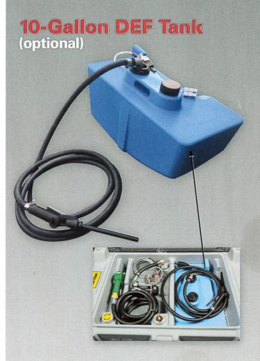
This 10-gallon capacity tank makes it easy to carry and dispense DEF fluid along with diesel fuel. The JDI-DEF10 Diesel Exhaust Fluid tank is molded out of rugged polyethylene and is designed to fit in the storage compartment of the 106-gallon Carrytank. It is a self-contained tank that includes a separate 12 volt pump, dispsensing hose and nozzle. It is powered by the same 12 volt source as the Carrytank with a separate power plug. No additional power cables are required.
